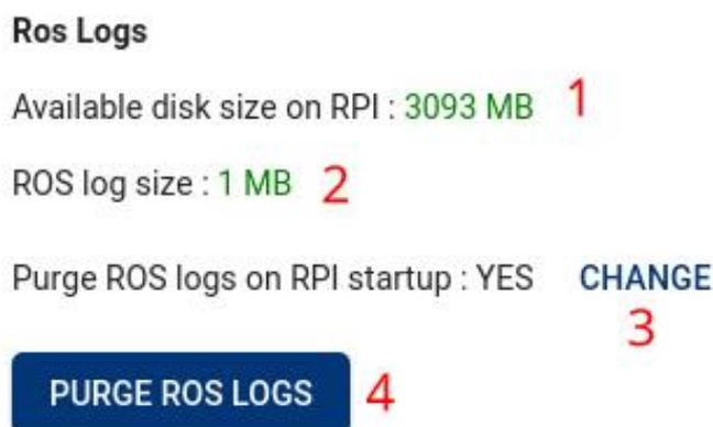
1. Available disk size on Raspberry Pi 3B. If the number is displayed in orange or red, it means that there is not enough space on the micro SD card.
