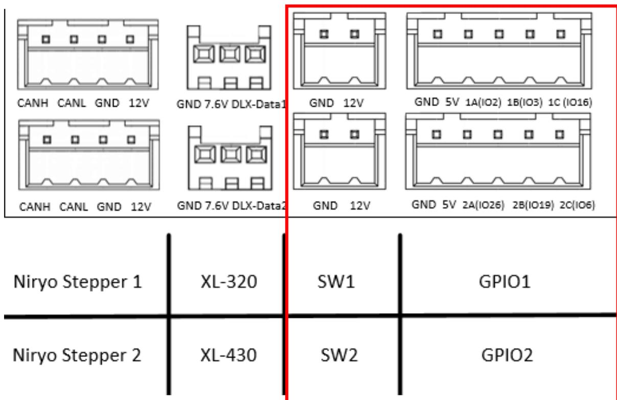
“SW1” and “SW2” connector can be used to plug a fan, a motor, etc.
