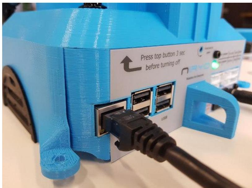
You can also use an Ethernet cable to physically connect your robot with your computer. This can be useful for example when you are in a Wi-Fi saturated location (exhibition, event, etc.).
