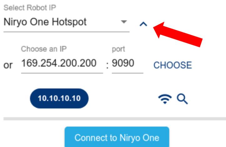
Write "169.254.200.200" (static IP) and click on "Choose" to select the IP address. Note that selecting the IP address just means that this IP will be used by Niryo One Studio, it does not mean that you are connected to the robot.
