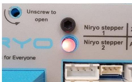
**!** Do not unplug or power off the robot now, you may damage the Raspberry Pi 3B inside the robot, or the micro SD card inside the Raspberry Pi 3B.
