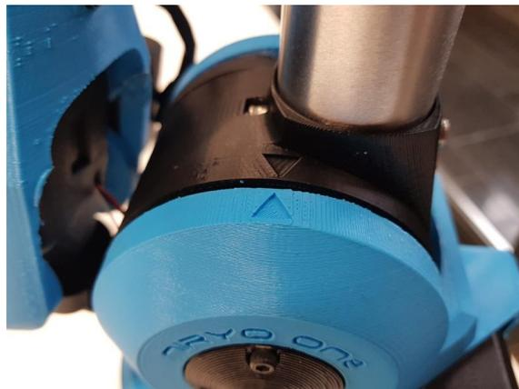
**⚠** Make sure that the mechanical parts are correctly lined up (+/- a few degrees), if the difference is too big you'll get an unwanted offset on some axis.
