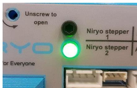
**i** Once the LED is blue or green, it means that the robot is fully started and you can start using it.
